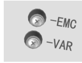
Schematic Diagram of Stop Screws for Iron Enclosure Cabinet
