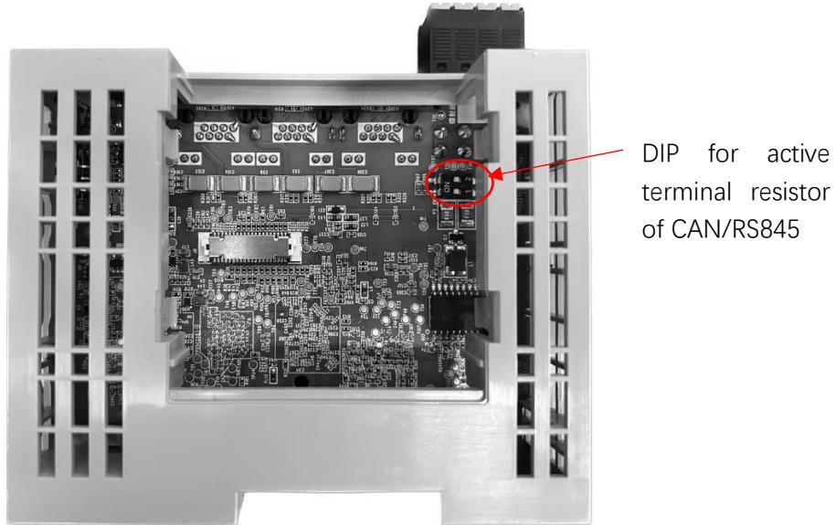
terminal resistance and DIP channel is shown in the table below.
