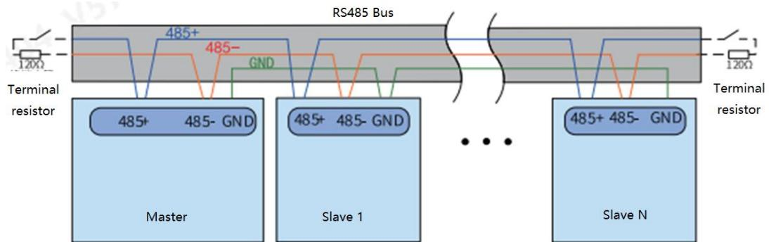
When fixing cables, do not bundle them together with AC power cables, high-voltage cables, etc. to avoid interference with communication signals.
