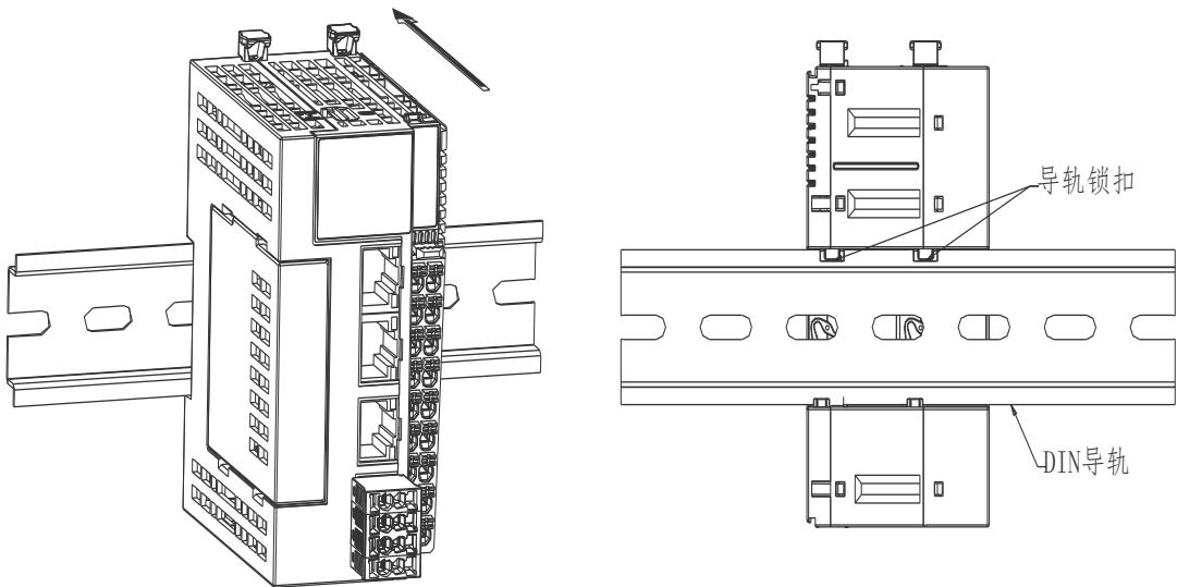
2. Confirm that the DIN rail lock of the host is in the locked state. The locked and unlocked states of the rail lock are shown in the figure below.
