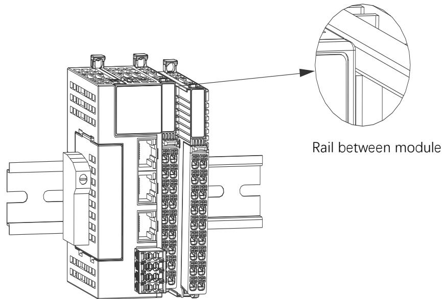
Install a DIN rail clip at each end of the main unit or module. When installing the rail clip, hook the bottom of the rail clip to the bottom of the rail and then rotate the rail clip so that the upper end of the rail clip hooks the upper end of the rail, and finally tighten the screws to lock the rail clip, as shown in the figure below.
