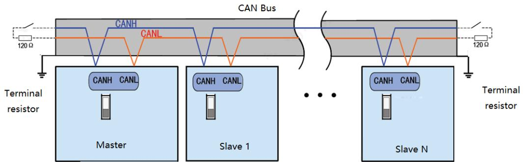
It is recommended to use shielded twisted pair cables for CAN bus connection. Two  $120\Omega$  terminal matching resistors are connected at both ends of the bus to prevent signal reflection. The shielding layer is generally reliably grounded at a single point. When fixing the cables, do not bundle them together with AC power cables, high-voltage cables, etc. to avoid interference with communication signals.
