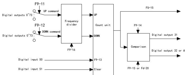
Note: In quadrature counting mode (Fd-19=1), encoder channels A and B are fixed as the UP and DOWN command channels.
