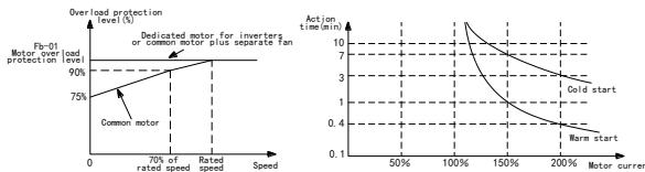
When the motor overload protection takes effect, the motor can continue to run only after it is cooled.
