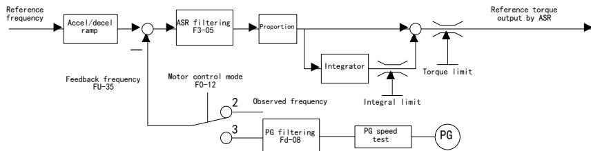
ASR structure (for PG V/F control) is as follows:
