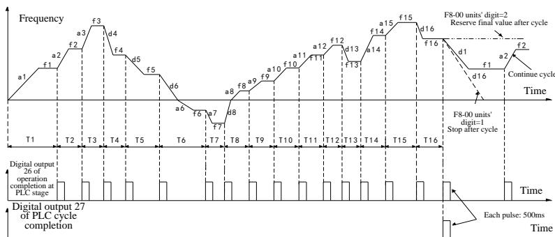
When the digital input 23 is valid, PLC operation pauses; when it is invalid, PLC operation restarts from the stage before the pause (start mode is determined by F1-19), as shown below.
