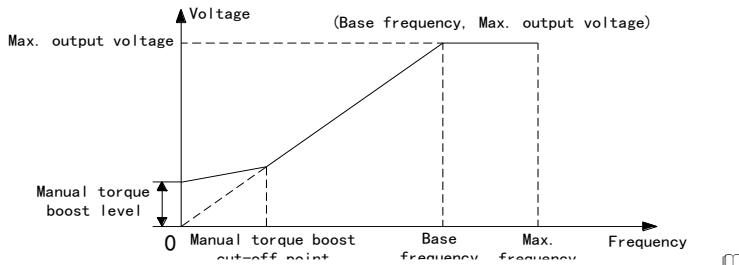
Auto torque boost can alter the voltage according to the load current, compensating for the voltage loss of the stator impedance and adapting to various load conditions automatically. It ensures a large output torque under heavy load and a small output current under no load.
