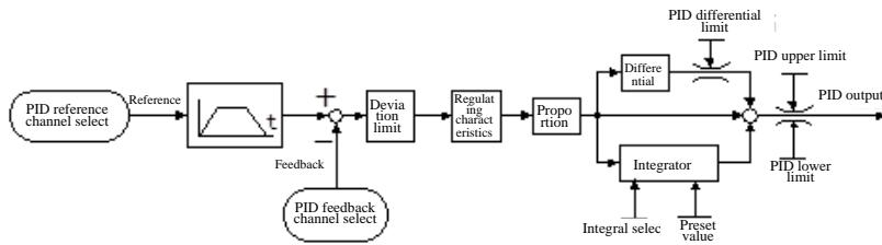
Process PID has three types of correction mode: reference frequency correction prior to accel/decel, reference frequency correction after accel/decel, and torque correction. These correction modes make it convenient to use the inverter in master-slave synchronous control and tension control.
