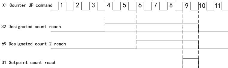
■ F9-16: count after combining input pulse and combine one count pulse via F9-16 pulse.
