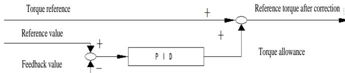
Free PID function: PID acts as a programmable module. Its input and output can be defined separately. PID output can be connected to the analog output.
