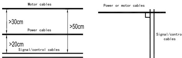
The longer the motor cables or the larger the section area of motor cables, the larger the ground capacitance, and the stronger the mutual coupling and disturbance. Therefore, the cables with specified section area and minimum length should be used.
