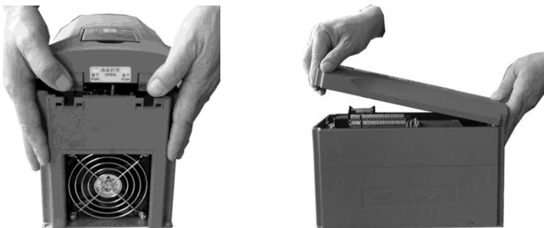
During uninstallation, disassemble keypad and press the two buckles on the top of cabinet simultaneously with two hands as shown in the left figure to take cover board down with slight upward force.
