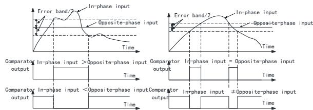
□ The result of comparison between two signals can be used as the trigger signal of inverter protection actions. Required protection actions can be selected according to hundred digit of "comparator configuration".
