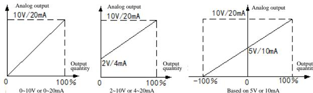
Adjusting the gain and bias can change the measuring range and correct the zero point. The calculation formula is:  $Y=X \times \text{gain} + \text{bias}$  ( $X$  is any item in the table of analog output functions).
