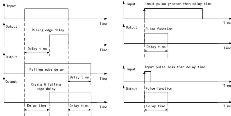
□ Using the timer can eliminate the signal jitter. Take the function of “rising edge delay” as an example, if the input pulse is shorter than the delay time, no signal will be output.
