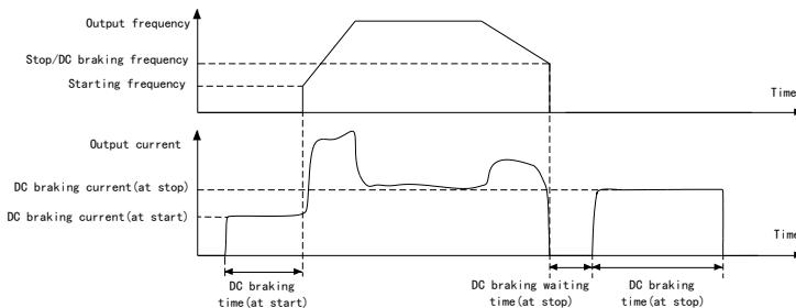
**Caution:** For high-speed or large-inertia loads, it is recommended to adopt “starts from searched speed” instead of “starts from starting frequency after DC braking”.
