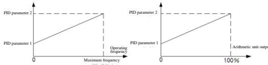
Principle of PID parameter regulation: first raise the proportional gain from a smaller value(e.g. 0.20) until the feedback signal starts oscillating, then lower it by 40~60% to stabilize the feedback signal; reduce the integral time from a larger value(e.g. 20.00s) until the feedback signal starts oscillating, then raise it by 10~50% to stabilize the feedback signal. Differential action can be introduced if there is a high requirement for overshoot and dynamic error.
