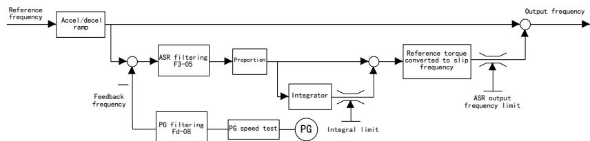
Note: In PG V/F control, if F3-07=0, ASR is limited by F3-10; if F3-07≠0, ASR limit= F3-10×F3-07÷2.5.
