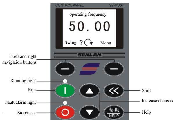
Basic hierarchical structure of LCD keypad is as follows:
