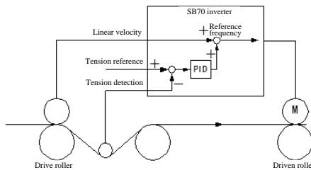
**Reference frequency correction after accel/decel:** PID output is added to the reference frequency after accel/decel. Unlike the previous correction mode, this mode can also perform the correction during accel/decel.
