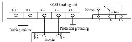
Wire between braking unit and inverter and braking resistor shall be within 5m, with minimum surrounded loop area.
