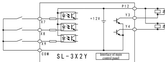
The digital I/O expansion board provides multi-channel inputs and outputs. The number of the channels can be decided by the user, for example, 5 channels of digital input (SL-5X), 5 channels of digital output (SL-5Y) and 3 channels of digital input plus 2 channels of digital output(SL-3X2Y).
