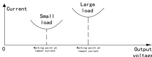
■ Auto energy-saving operation is only valid for V/F control and only applicable to applications with a stable load.
