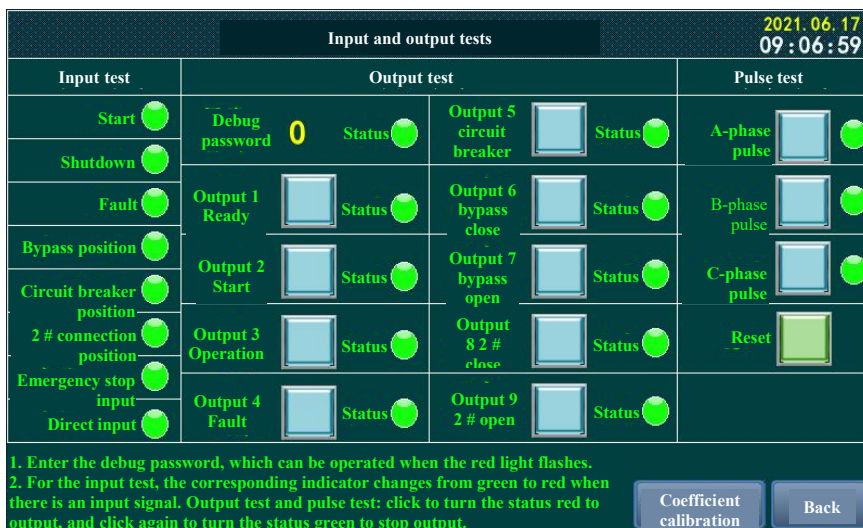
Fig. 4.15 Input and Output Tests
